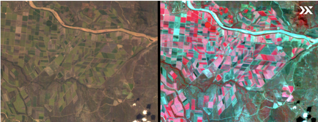
The power of HSI becomes apparent when compared with multispectral imaging. The hyperspectral image (right) highlights the superior level of detail, capturing vast information beyond what is possible with MSI (left). This capability enables precise pest detection and analysis, invasive species and disease detection, soil health and nutrient content determination, and chlorophyll content, empowering farmers with comprehensive insights for efficient decision-making in precision agriculture.
