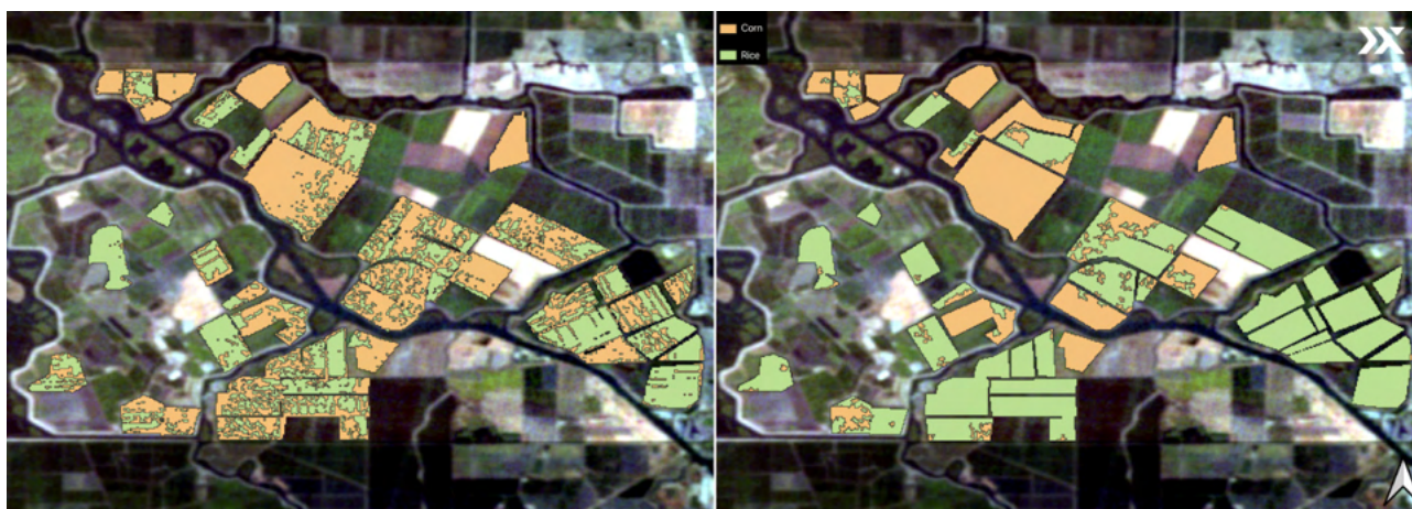
Analysis of rice and corn fields over Central Valley, California (U.S.A.) shows the power of hyperspectral imagery (right) over multispectral imagery (left) in distinguishing species. When validated with ground-truth datasets from the USDA 2023 Crop Map, hyperspectral imagery had an overall classification accuracy of 91% compared to the 65% accuracy using seven bands from Landsat (30 m) imagery.
